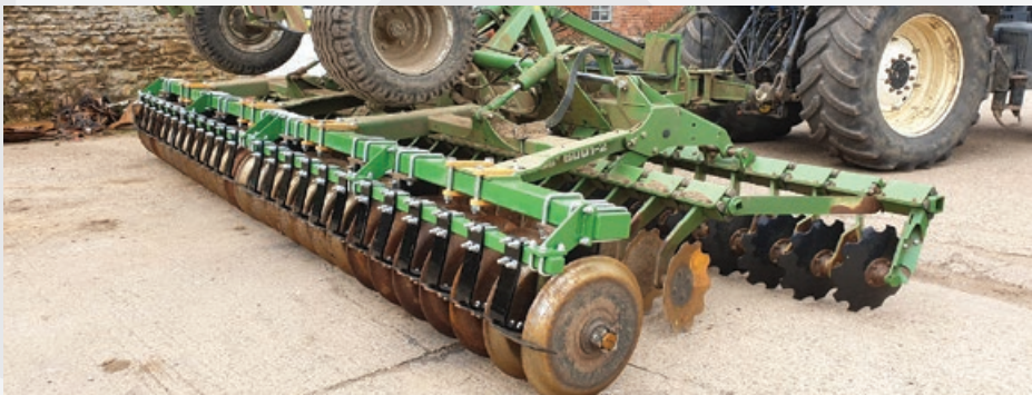
575mm U-Shaped Open Soil Packer
